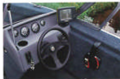
The console features a Humminbird® fishfinder, tachometer and fuel gauge. The 170 and 190 also include a speedometer and voltmeter.
