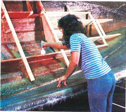
apply extra layers of woven roving. And we actually put string glass in the bottom the strakes – that means no air bubbles – and then reinforce the strakes with a combination of woven roving and mat glass. Did you know that some boat companies actually fill their strakes – the main component for linear strength in the hull – with PUTTY?
