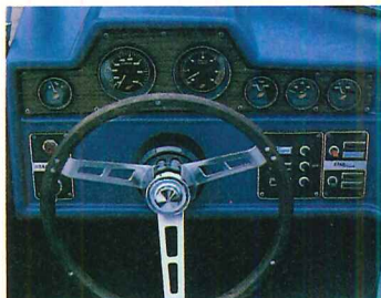
Command Instrumentation includes tach, speedometer, amp. meter, fuel tank and oil light. Temp gauge and trim indicator on I.O. models.
