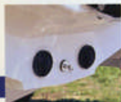
Performance pad on stepped hull to improve performance characteristics
