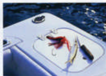
Rear deck with hawse pipes for rear cleats to eliminate any on-deck obstructions, an insulated baitwell with composite cutting board lid, and stainless steel rod holders
