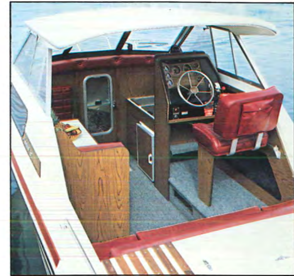
Cockpit of the American 22 Express showing fully instrumented controls and galley area.
